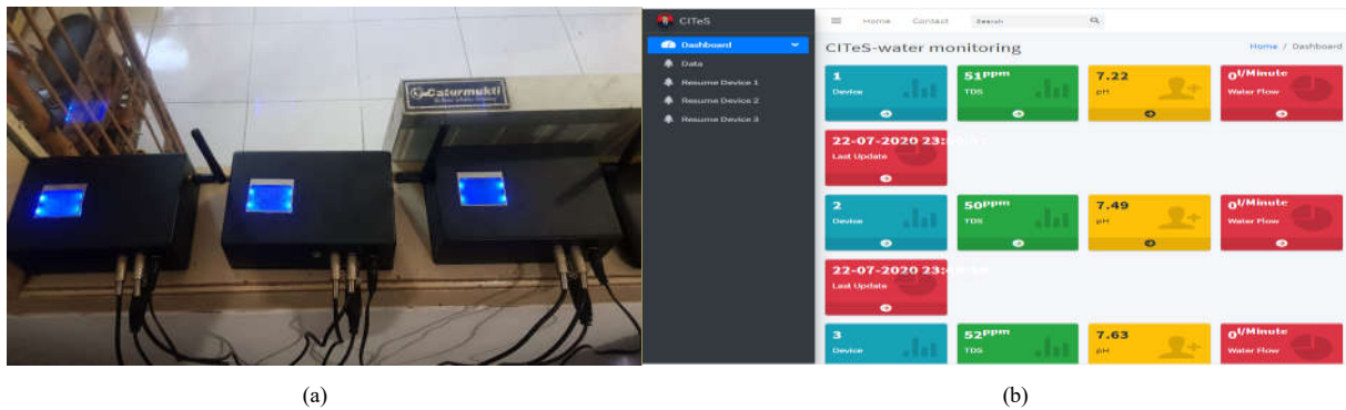
Fig. 5. The system integration (a), and the web-base monitoring system (b).
