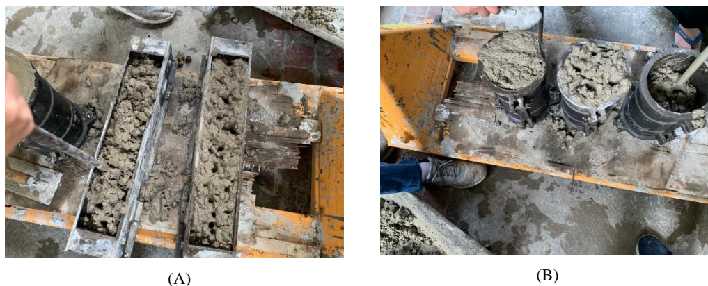
Figure 1. (a) manufacture of concrete specimen of flexural strength test (b) manufacture of concrete specimen of flexural strength test
