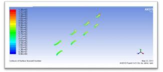
Fig. 8. The contour of Nusselt number for 1.7 mm spacing in an aligned arrangement
