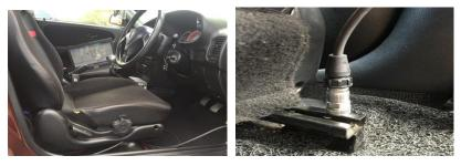
Fig. 4. Accelerometer attached on the car seat.
