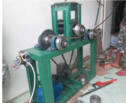
Gambar 8. Alat roll pipa besi
